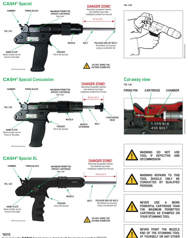
Every tool in the CASH® Special range is stamped with the maximum permitted (PROOF) cartridge, showing the maximum grains (GRN) that should be used
