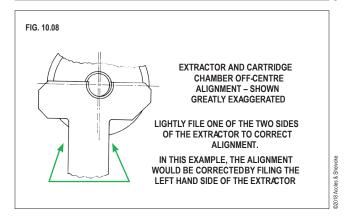
It should only be necessary to remove a very small amount of material from the extractor when fitting it. Any rough filing or excessive removal of material could cause poor extraction or burst cases.
